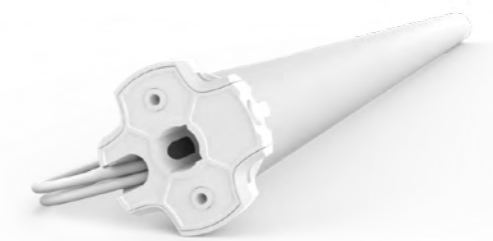
Automate Wire-Free Li-ion Q3.0 5V, 3.0Nm, Ø35mm, 20-28PRM, 849mm long
